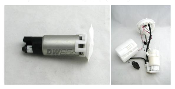
6 – install the assembly into the bucket and check to make sure all connectors are installed and wires are tucked in place, reinstall the vertical support retainers
