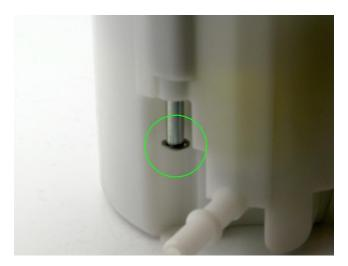
2 – to remove the center section of the assembly from the bucket, there are 2 spring tabs and 1 clip. While pulling on the center section of the assembly, lift the middle tab (black circle) and squeeze the outside tabs together (green circles). Once all 3 tabs and clip are loosened, separate the center assembly from the bucket
